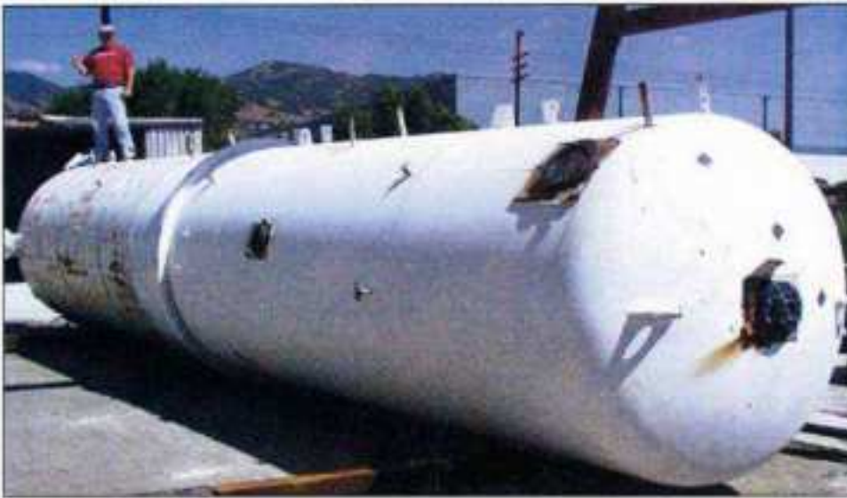
Vacuum degasifier 11 Meters long X 2 Meters diameter KYNAR 2850 PC coated internally by FisherMoore, North Salt Lake City, Utah for a major chip manufacturer to provide purity and reliability.
